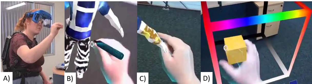
Figure 1: We present 3DCoLAR, an art application that aims to explore painting 3D models and color selection approaches. A) A user wearing an AR HMD, B) can use either a virtual pen or C) their fingertip. D) We also expand typical 2D color picker interfaces, allowing for 3D space representation of color spaces.
