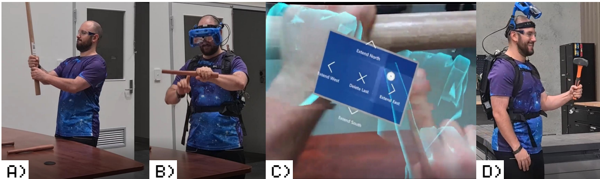
Figure 1: Figure 1: We introduce B-Handy, a system that supports the usage of bio-mechanics as a means of measuring every day objects. In our example: A) A user is confused, unable to determine the right handle length for a hammer. B-C) The user interacts with the B-Handy UI to create virtual copies of their hand to aid in bio-mechanical measurements. D) The result of our system enables the user to rapidly infer measurements of every day tools through this process.
